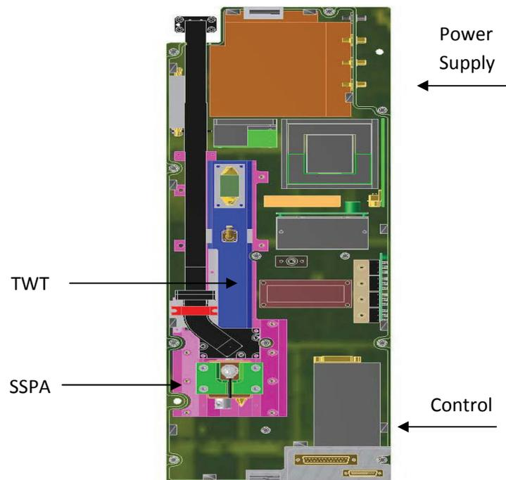
Figure B. An Amplifier Example
