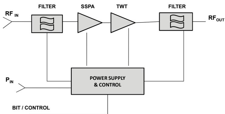
Figure A. Typical TWT Amplifier Block Diagram
